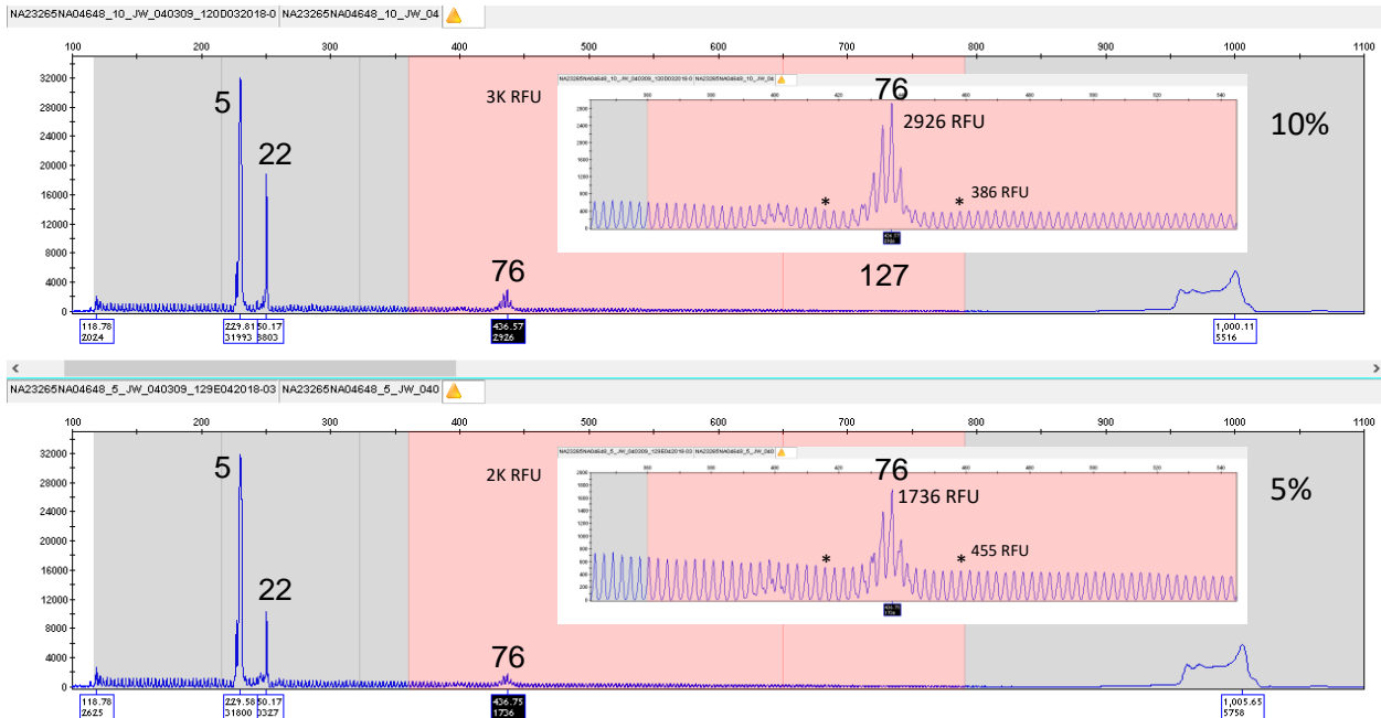
Figure 17. Limit of detection for mosaicism tested by mixing NA23265 (12, 63, 76) at a mass allele fraction of between 1% and 50% into a background of NA04648 (5, > 200). Shown are both 5% and 10% samples. The * represents \pm 7 repeats from the called peak.
