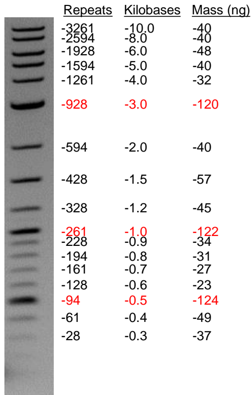
Figure 12. New England Biolabs® Quick-Load 1 kb Plus DNA Ladder Sizing conversion from Kilobases to Repeats.
