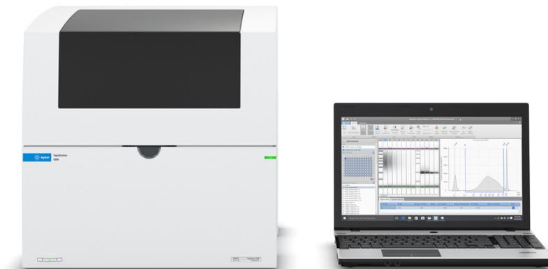
For the Agilent 4200 TapeStation system, a portfolio of ScreenTape assays is available. The credit card-sized, disposable ScreenTape device carries multiple separation lanes for analyzing DNA and RNA samples. Each ScreenTape device has 16 lanes so that each sample is analyzed in an individual lane, completely eliminating contamination and carryover.
