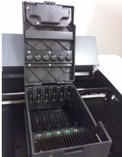
Figure 7 Slots for the optical modules
