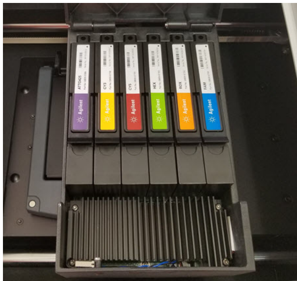
Figure 10 Installed optical modules
